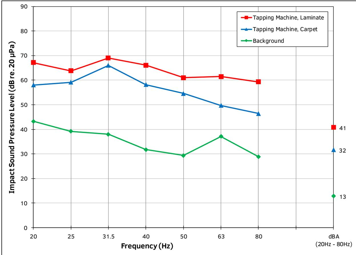
**Figure 6 – Plot of measured tapping machine impact sound pressure levels.**
