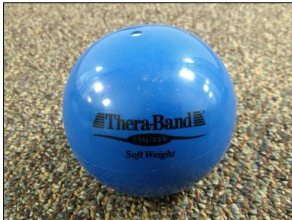
**Figure 3 – Photo of the ball drop source.**
