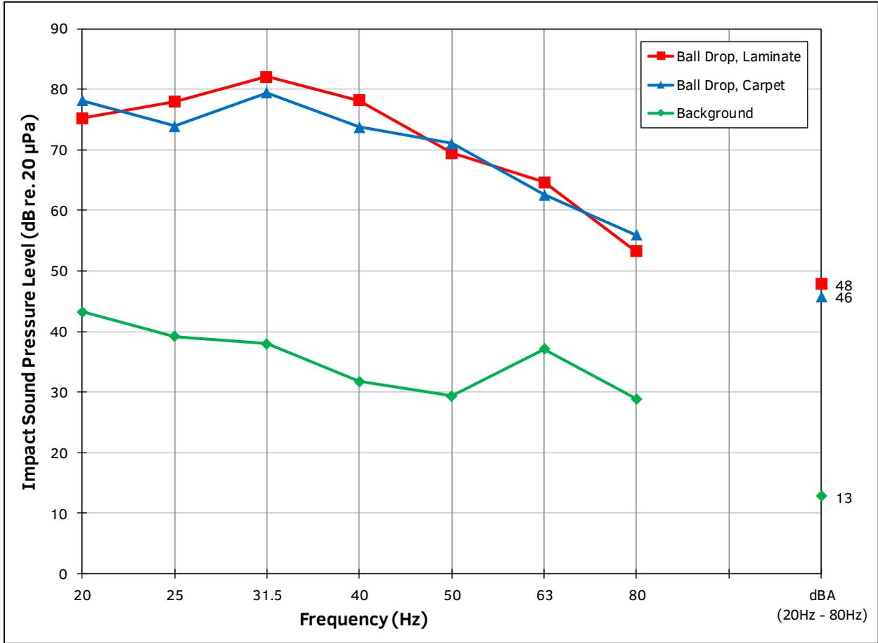
**Figure 4 – Plot of measured ball drop impact sound pressure levels.**
