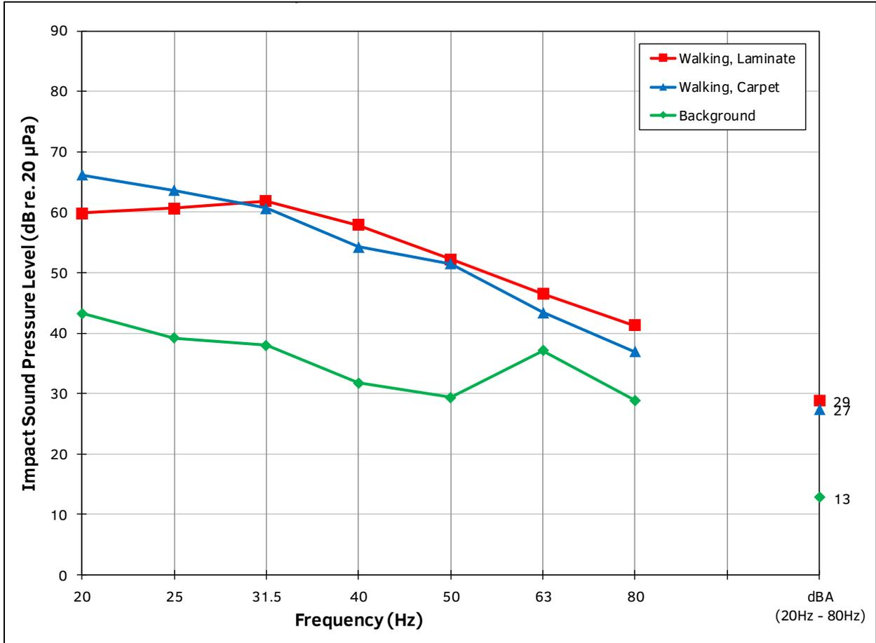
Figure 2 – Plot of measured walker impact sound pressure levels.
