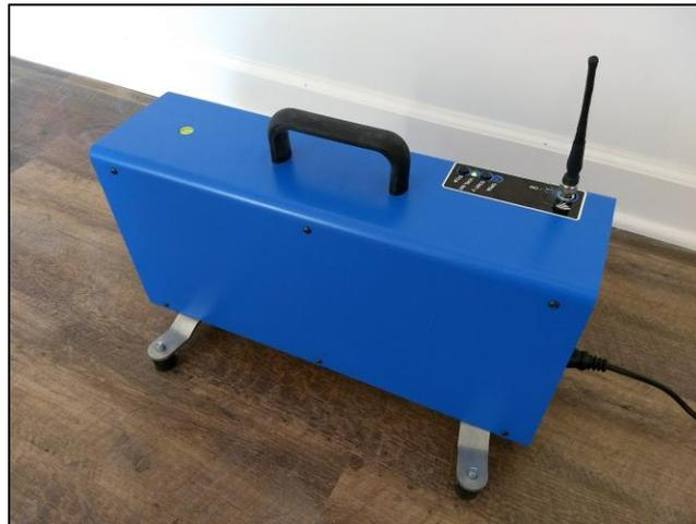
**Figure 5 – Photo of the tapping machine source.**
